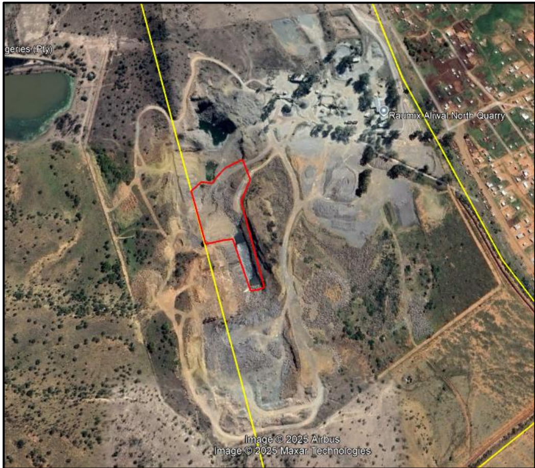
Figure 7: Satellite image of the bridge being added and dam/sump being refilled (red polygon) where the yellow polygon indicates the “original” mining boundary.
