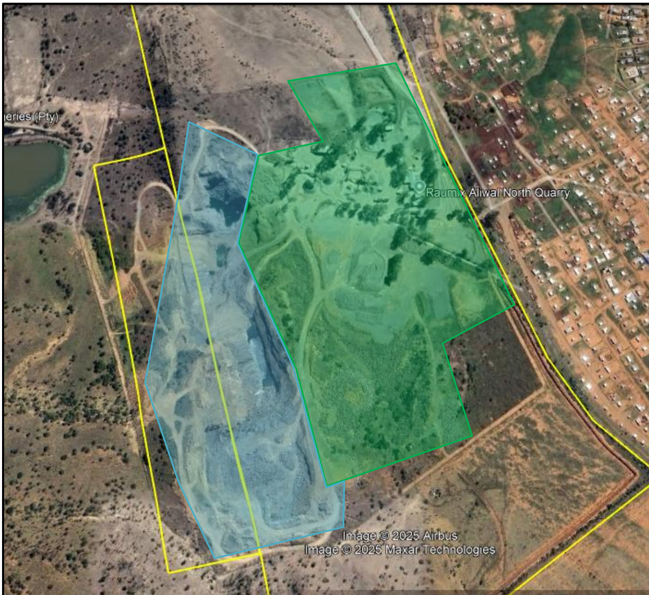
Figure 8: Satellite image of the processing and associated mining areas (green shaded polygon) that will be developed for grazing purposes, and the quarry pit (blue shaded polygon) to be rendered safe and left as a landscape feature.
